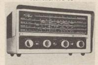
1958-Still Marketed. Frequency Coverage: .54 to 31.0 mc; (1) .54 to 1.6 mc. (2) 1.6 to 4.5 mc. (3) 4.0 to 12.0 mc. (4) 10,5 to 31.0 mc Specifications: 4 tubes plus rectifier; un-balanced antenna input; 455 kc if; operates on 115 v, 50/60 cycle ac or dc line. Special Features: Internal speaker; electrical bandspread and receive-standby switch.
